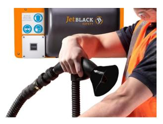
If you're worried that blower driven air isn't as powerful as compressed air, rest assured. Blower driven air creates a steady flow of air to dislodge most dust, fibres and particles from workers', their clothing, and their equipment, and can be used to generate an air shower or air curtain. This is the experience of de-dusting in a personnel cleaning booth (taking an 'air shower').
